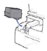
☐ If you are removing the color cartridge (either the BC-61 Color BJ Cartridge or BC-62 Photo BJ Cartridge), pull up on the right cartridge to remove it.
