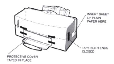
☐ If the protective cover is not available, you can use a piece of heavier-weight paper (such as card stock). Cut the paper so that it covers the paper output slot.
