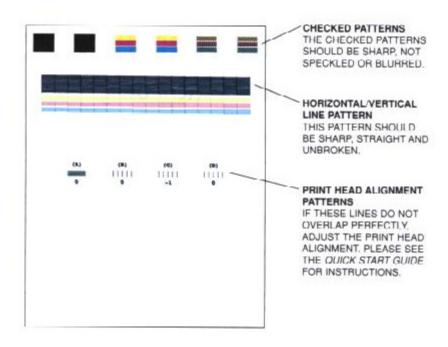
If any portion of the Nozzle Check Pattern is incorrect, clean the print head. See the next section for details.
