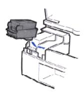
☐ Insert the BJ cartridge slightly diagonally into the holder. Make sure the cartridge is aligned with the guides, then press down on the cartridge at the circle mark to lock it in place.
