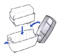
☐ If necessary, open a new BJ cartridge box. Then remove the cap and tape.
